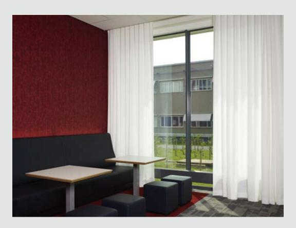
The fullness and wave depth of the curtain depends on the selected glider cord and the applied spacing between the curtain hooks. The stack depth varies between 8cm and 14cm.
